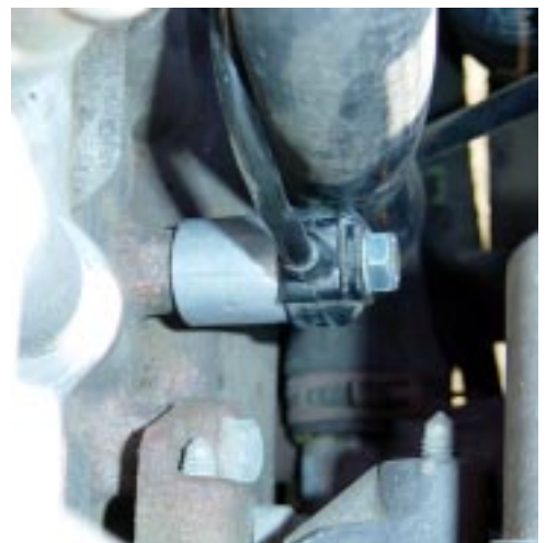
Knock Sensor with bushing installed.
